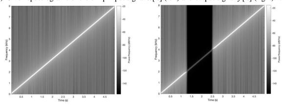
(a) Given spectrograms of the chirp input signal x[n] (left) and output signal y[n] (right). 7 points.
