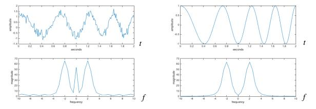
Design a second-order infinite impulse response (IIR) filter to filter the acquired signal above on the left to give the sinusoidal signal above on the right. Filter should be bounded-input bounded-output stable.
